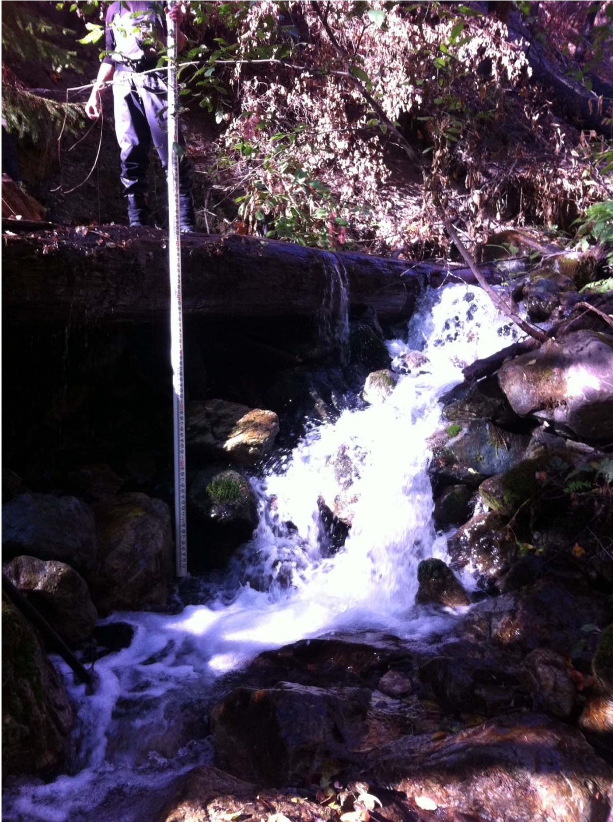
Photo 3. Falls with 6 ft height and >2 ft lateral with not jump pool at base.
